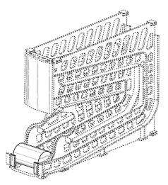
The Figure of the '646 patent is this perspective view of a gravity feed dispenser display. *Id.* As depicted, certain elements in the front area of the design are drawn in solid lines, but much of the rearward structure is illustrated by broken lines. The Description of the invention explains:
